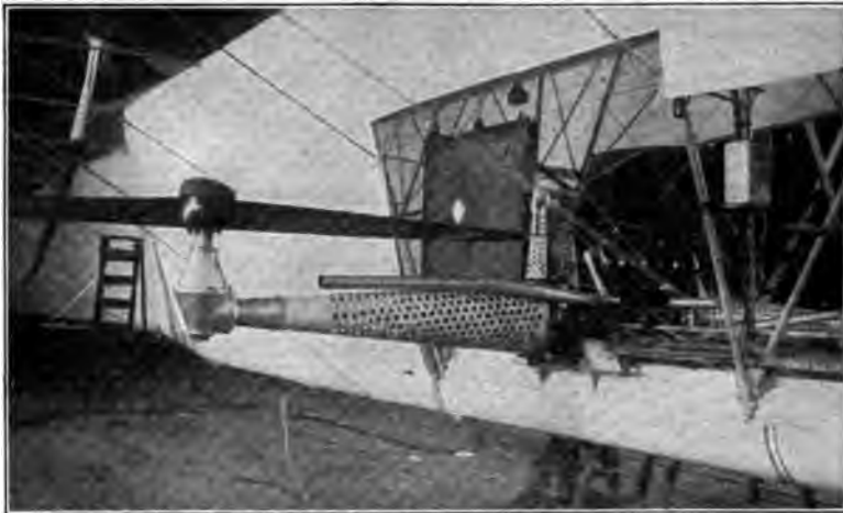
Fig. 26. View of Rear Propellers Set Horizontally for Lifting the Airship
